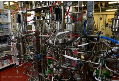
OSCAR bi stage bioreactor with membrane recycling
