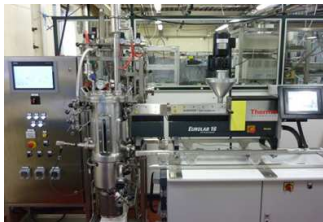
Innovative Bioprocess: HDMB Bioextrusion-fermentation bioreactor
